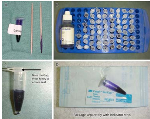
Fig 1. Gentian violet marking system. Labeled microcentrifuge tube and two round, wood toothpicks. Cotton tip applicators with wood end shaved to a fine point may also be used (A). Microcentrifuge tube rack may be used to facilitate preparation of multiple tubes for autoclaving (B). The cap should be pressed firmly to ensure a tight seal (C). The tube may be packaged separately (D). for autoclaving in case a spill does occur.
