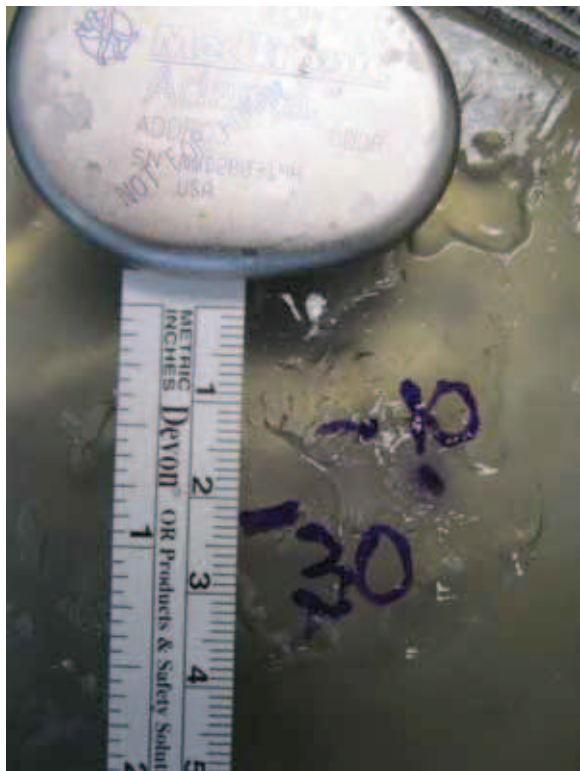
Figure 2. Distance of Hyfrecator wand to a pacemaker device, causing atrial inhibition at both “normal use” of 10W and High setting of 30W
